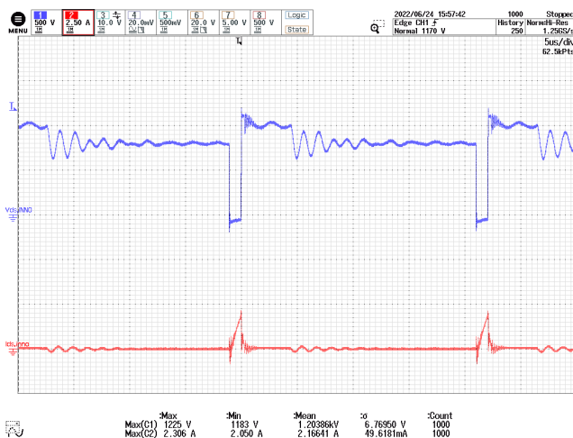
Figure 51 – InnoSwitch3-AQ Drain Voltage and Current. 800 V DC , 2.333 A Load, 85 °C Ambient. CH1: V_{DS(IC1)} , 500 V / div. CH2: I_D(IC1) , 2.5 A / div. Time: 5 μs / div.
