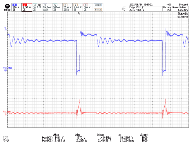
Figure 52 – InnoSwitch3-AQ Drain Voltage and Current. 1000 V DC , 2.333 A Load, 85 °C Ambient. CH1: V_{DS(IC1)} , 500 V / div. CH2: I_D(IC1) , 2.5 A / div. Time: 5 μs / div.
