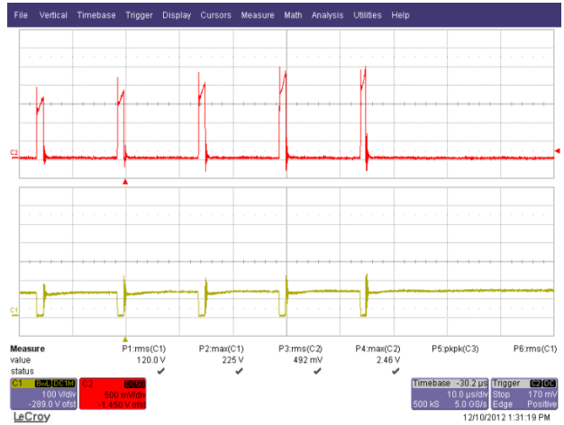
Figure 52 – 90 VAC, 60 Hz Start-up. Upper: I_{DRAIN} , 500 mA / div. Lower: V_{DRAIN} , 100 V, 10 \mu s / div.
