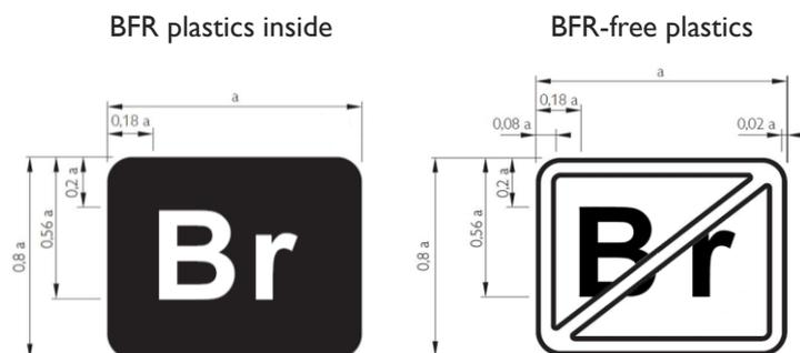
The dimension of “a” shall be greater than 9 mm and the typeface to be used is ‘Gill Sans serif’.
