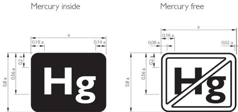
The dimension of “a” shall be greater than 9 mm and the typeface to be used is ‘Gill Sans serif’.
