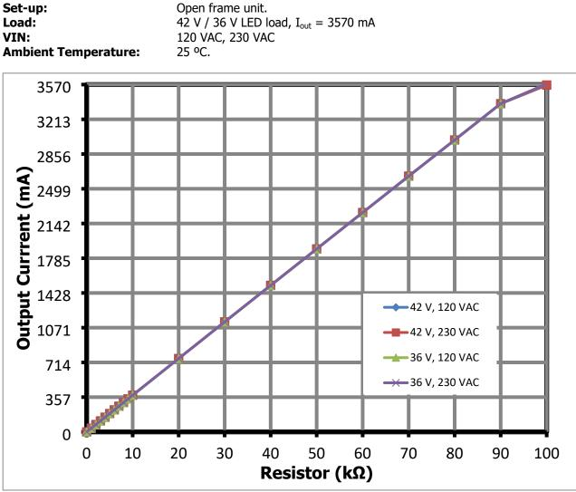
Figure 37 – 0 – 100 k $\Omega\,$  Dimming Curve at 42 V & 36 V LED Load.
