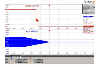
Figure 95 – Brown-in Test at 0.5 V / s. Upper:  $I_{OUTPUT}$ , 500 mA / div. Lower:  $V_{INPUT}$ , 100 V / div. Time Scale: 100 s / div.
