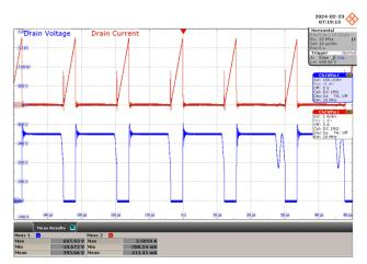
Figure 71 – 230 VAC, 42 V LED Load. Upper:  $I_{DRAIN}$ , 1 A / div. (Max = 605.93 V) Lower:  $V_{DRAIN}$ , 150 V / div. (Max = 3.51 A) Time Scale: 10 µs / div.
