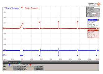
Figure 75 – 100 VAC, 42 V LED Load. Upper:  $I_{DRAIN}$ , 2 A / div. Lower:  $V_{DRAIN}$ , 150 V / div. Time Scale: 20 µs / div.
