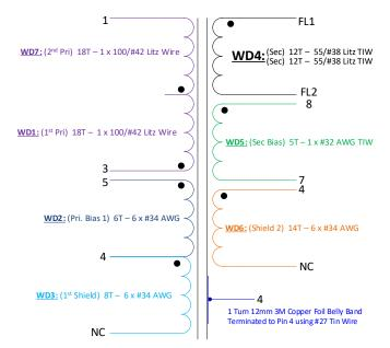
**Figure 21** – Transformer Electrical Diagram.
