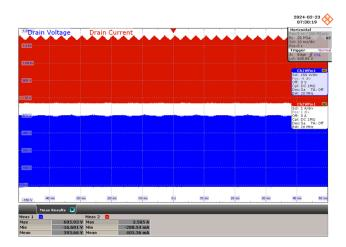
$\begin{array}{l} \textbf{Figure 70-230 VAC, 42 V LED Load.} \\ \textbf{Upper: } I_{DRAIN}, 1 \text{ A / div. (Max = 605.93 V)} \\ \textbf{Lower: } V_{DRAIN}, 150 \text{ V / div. (Max = 3.59 A)} \\ \textbf{Time Scale: } 10 \text{ ms / div.} \end{array}$
