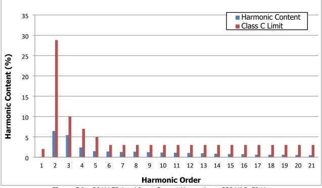
Figure 34 – 36 V LED Load Input Current Harmonics at 230 VAC, 50 Hz.
