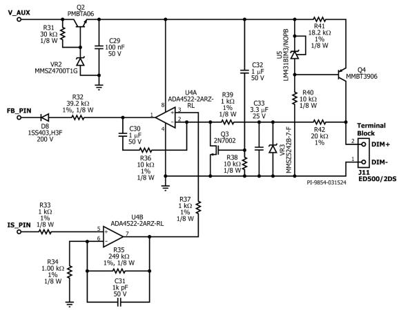
Figure 6 – Schematic, Dimming Section.
