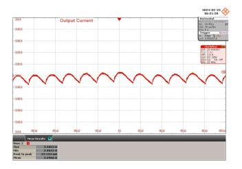
Figure 84 – 230 VAC, 42 V LED Load.  $$I_{OUTPUT}$, 20 mA / div., 20 <math display="inline">\mu s$  / div.
