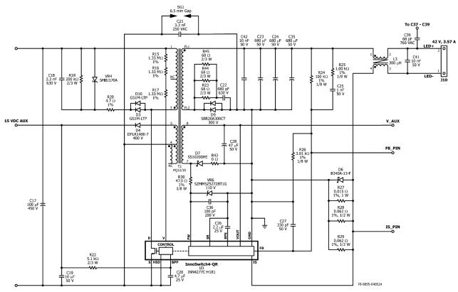
Figure 5 – Schematic, DC-DC Flyback Section.
