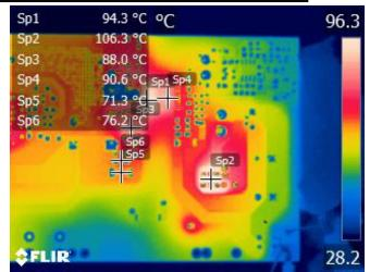
Figure 41 – 100 VAC 60 Hz, Full Load. InnoSwitch4-QR IC (U3), Output Diode Snubber Resistors (R23, R44, R45).
