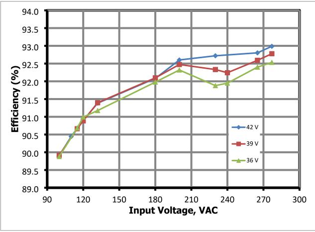
Figure 27 – Efficiency vs. Line and LED Load.
