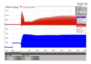
Figure 62 – 100 VAC, 42 V LED Load. Upper:  $I_{DRAIN}$ , 2 A / div. (Max = 422.13 V) Lower:  $V_{DRAIN}$ , 150 / div. (Max = 5.51 A) Time Scale: 100 ms / div.
