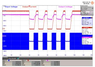
Figure 88 – 230 VAC, 42 V LED Load. 1 s On – 1 s Off. Upper:  $I_{OUT}$ , 1 A / div.  $V_{OUT}$ , 10 V / div. Lower:  $V_{IN}$ , 200 V / div., 2 s / div.
