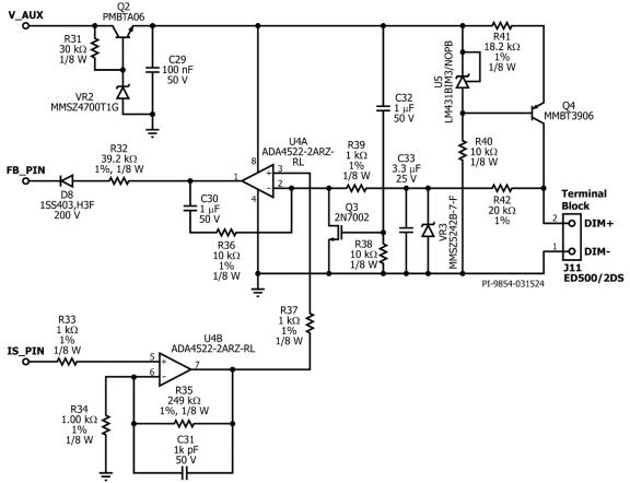
**Figure 9** – 3-Way Dimming Schematic.
