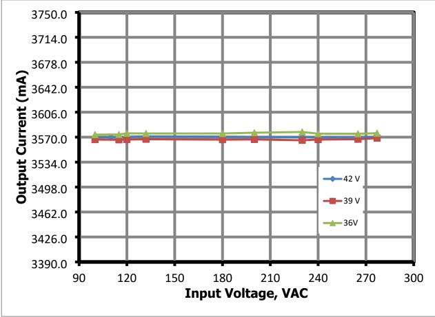
Figure 28 – Current Regulation vs. Line and LED Load.
