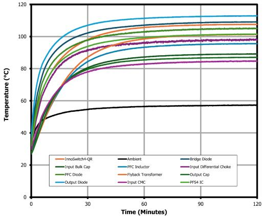
Figure 45 – Component Temperature at 55°C Ambient - Open Frame (100 VAC, 42 V LED load).
