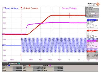
Figure 53 – 277 VAC, 42 V LED, Output Rise. Upper: V<sub>OUT</sub>, 20 V / div, I<sub>OUT</sub>, 1 A / div. Lower: V<sub>IN</sub>, 300 V / div., 200 ms / div. Turn on Time: 642 ms
