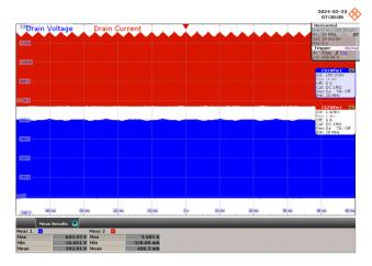
Figure 68 – 120 VAC, 42 V LED Load. Upper:  $I_{DRAIN}$ , 1 A / div. (Max = 605.93 V) Lower:  $V_{DRAIN}$ , 150 V / div. (Max = 3.56 A) Time Scale: 10 ms / div.
