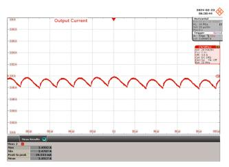
Figure 83 – 120 VAC, 42 V LED Load.  $$I_{OUTPUT}$, 20 mA / div., 20 <math display="inline">\mu s$  / div.
