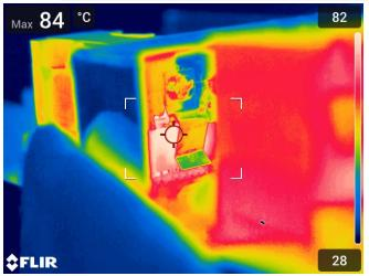
**Figure 40** – 100 VAC 60 Hz, Full Load. HiperPFS-4 IC (U2).
