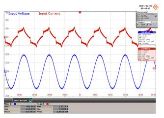
$\label{eq:Figure 49-277 VAC, 42 V LED Load.} \\ Upper: I_{IN}, 1 \text{ A / div.} \\ Lower: V_{IN}, 200 \text{ V / div.}, 10 \text{ ms / div.} \\ \end{aligned}$
