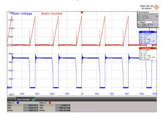
Figure 69 – 120 VAC, 42 V LED Load. Upper:  $I_{DRAIN}$ , 1 A / div. (Max = 605.93 V) Lower:  $V_{DRAIN}$ , 150 V / div. (Max = 3.47 A) Time Scale: 10 µs / div.
