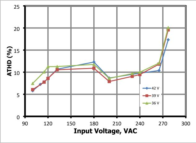
**Figure 30** – %ATHD vs. Line and LED Load.
