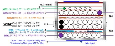
Figure 22 – Transformer Build Diagram.
