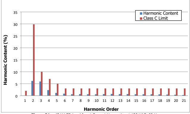
Figure 31 – 42 V LED Load Input Current Harmonics at 120 VAC, 60 Hz.
