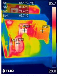
Figure 43 – 100 VAC 60 Hz, Full Load. PFC Diode (D2), Bridge Diode (BR1), Input Differential Inductor (L2), PFC Inductor Core (T1).
