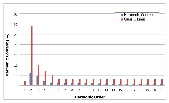
Figure 32 – 42 V LED Load Input Current Harmonics at 230 VAC, 50 Hz.
