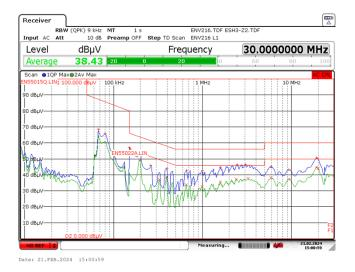
Figure 92 – Conducted EMI, Floating Output. 230 VAC, 42 V Full Load LED. Passed.
