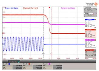
Figure 57 – 277 VAC, 42 V LED, Output Rise. Upper: V<sub>OUT</sub>, 20 V / div, I<sub>OUT</sub>, 1 A / div. Lower: V<sub>IN</sub>, 300 V / div., 100 ms / div. Turn off Time: 85 ms
