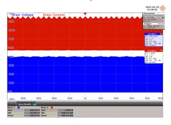
Figure 72 – 277 VAC, 42 V LED Load. Upper:  $I_{DRAIN}$ , 1 A / div. (Max = 605.93 V) Lower:  $V_{DRAIN}$ , 150 V / div. (Max = 3.59 A) Time Scale: 10 ms / div.
