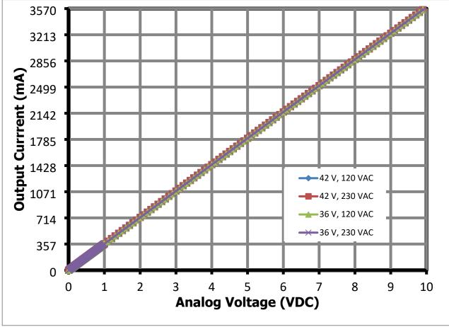
Figure 36 – 0 V – 10 V Dimming Curve at 42 V & 36 V LED Load.
