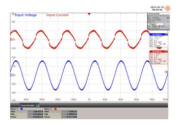
$\label{eq:Figure 48-230 VAC, 42 V LED Load.} \\ Upper: I_{IN}, 1 \text{ A / div.} \\ \text{Lower: } V_{IN}, 200 \text{ V / div.}, 10 \text{ ms / div.} \\ \end{aligned}$
