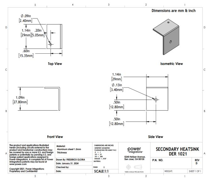
Figure 25 – Secondary Heat Sink Drawing.
