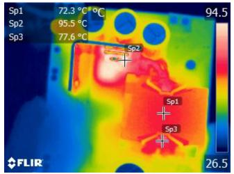
Figure 42 – 100 VAC 60 Hz, Full Load. Output Diode (D9), DC-DC Flyback Transformer Core (T2).
