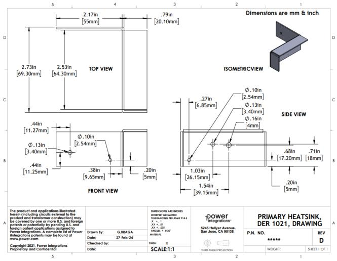
Figure 23 – Primary Heat Sink Drawing.
