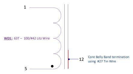
Figure 19 – PFC Inductor Electrical Diagram.
