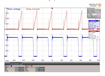
$\label{eq:Figure 73-277 VAC, 42 V LED Load.} \\ Upper: I_{DRAIN}, 1 \text{ A / div. (Max = 605.93 V)} \\ \text{Lower: V}_{DRAIN}, 150 \text{ V / div. (Max = 3.51 A)} \\ \text{Time Scale: 10 } \mu\text{s / div.} \\ \end{aligned}$
