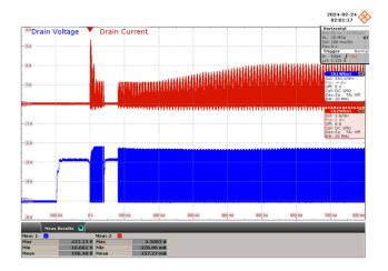
$\label{eq:Figure 64-230 VAC, 42 V LED Load.} \\ Upper: I_{DRAIN}, 1 \text{ A / div. (Max = 422.13 V)} \\ \text{Lower: } V_{DRAIN}, 150 \text{ / div. (Max = 3.31 A)} \\ \text{Time Scale: 100 ms / div.} \end{aligned}$
