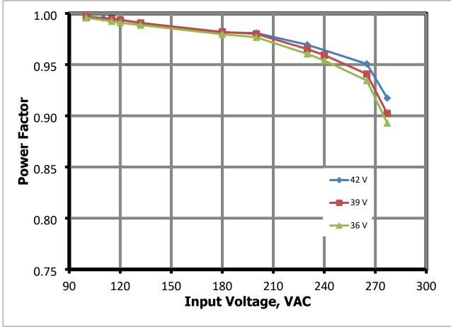
Figure 29 – Power Factor vs. Line and LED Load.
