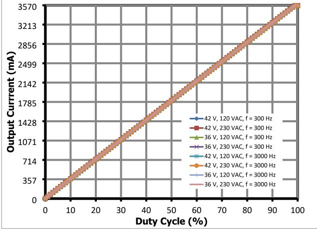
Figure 38 – Variable Duty PWM (f = 3000 Hz and 300 Hz) Dimming Curve at 42 V & 36 V LED Load.
