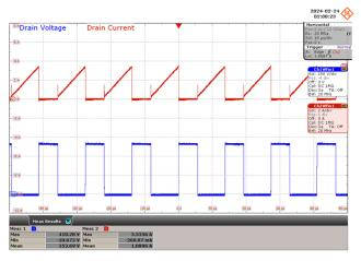
Figure 59 – 120 VAC, 42 V LED Load. Upper:  $I_{DRAIN}$ , 2 A / div. (Max = 410.28 V) Lower:  $V_{DRAIN}$ , 150 V / div. (Max = 3.53 A) Time Scale: 10 µs / div.
