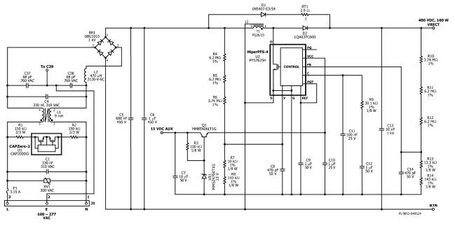
Figure 4 – Schematic, Input and PFC Section.
