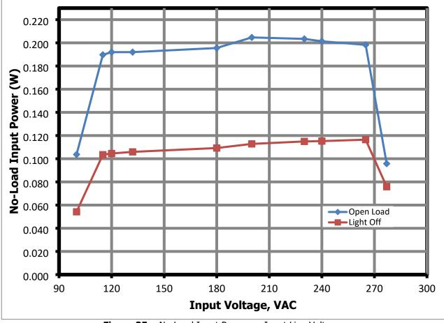
Figure 35 – No-Load Input Power vs. Input Line Voltage.
