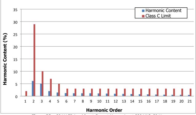
Figure 33 – 39 V LED Load Input Current Harmonics at 230 VAC, 50 Hz.
