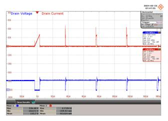
Figure 77 – 120 VAC, 42 V LED Load. Upper:  $I_{DRAIN}$ , 2 A / div. Lower:  $V_{DRAIN}$ , 150 V / div. Time Scale: 20  $\mu$ s / div.
