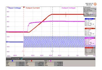
**Figure 52** – 230 VAC, 42 V LED, Output Rise. Upper: V<sub>OUT</sub>, 20 V / div, I<sub>OUT</sub>, 1 A / div. Lower: V<sub>IN</sub>, 300 V / div., 200 ms / div. Turn on Time: 652 ms
