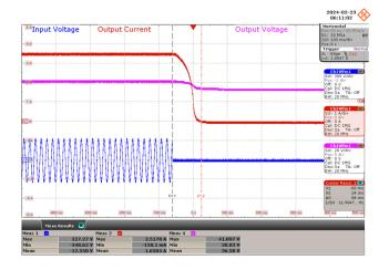
**Figure 56** – 230 VAC, 42 V LED, Output Rise. Upper: V<sub>OUT</sub>, 20 V / div, I<sub>OUT</sub>, 1 A / div. Lower: V<sub>IN</sub>, 300 V / div., 100 ms / div. Turn off Time: 84 ms
