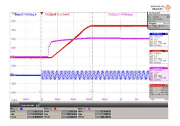
**Figure 50** – 100 VAC, 42 V LED, Output Rise. Upper: V<sub>OUT</sub>, 20 V / div, I<sub>OUT</sub>, 1 A / div. Lower: V<sub>IN</sub>, 300 V / div., 200 ms / div. Turn on Time: 648 ms
