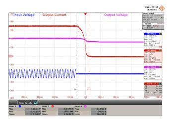
**Figure 54** – 100 VAC, 42 V LED, Output Rise. Upper: V<sub>OUT</sub>, 20 V / div, I<sub>OUT</sub>, 1 A / div. Lower: V<sub>IN</sub>, 300 V / div., 100 ms / div. Turn off Time: 85 ms
