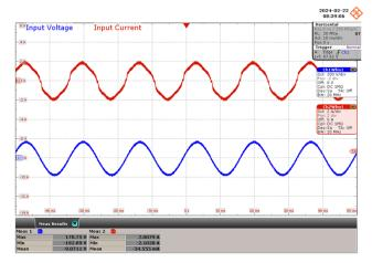
$\label{eq:Figure 47-120} \begin{array}{l} \mbox{I20 VAC, 42 V LED Load.} \\ \mbox{Upper: } I_{IN}, \mbox{ 2 A / div.} \\ \mbox{Lower: } V_{IN}, \mbox{ 200 V / div., 10 ms / div.} \end{array}$
