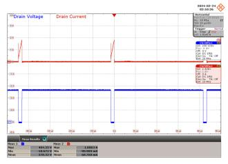
$\label{eq:Figure 61-277 VAC, 42 V LED Load.} \\ Upper: I_{DRAIN}, 1 \text{ A / div. (Max = 404.35 V)} \\ \text{Lower: } V_{DRAIN}, 150 \text{ V / div. (Max = 1.81 A)} \\ \text{Time Scale: } 10 \ \mu\text{s / div.} \end{aligned}$
