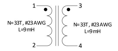
Figure 15 – CMC Electrical Diagram.
