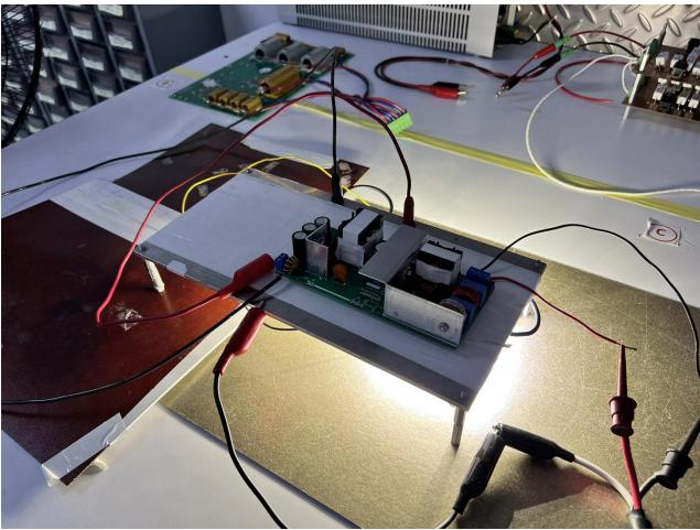
Figure 90 – Conducted EMI Test Set-up.
