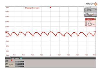
Figure 82 – 100 VAC, 42 V LED Load.  $$I_{OUTPUT}$, 20 mA / div., 20 <math display="inline">\mu s$  / div.
