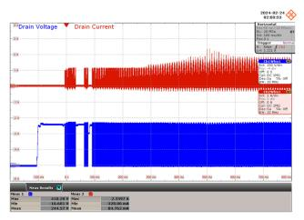
$\label{eq:Figure 65-277 VAC, 42 V LED Load.} \\ Upper: I_{DRAIN}, 1 \text{ A / div. (Max = 410.28 V)} \\ \text{Lower: } V_{DRAIN}, 150 \text{ / div. (Max = 2.36 A)} \\ \text{Time Scale: 100 ms / div.} \end{aligned}$
