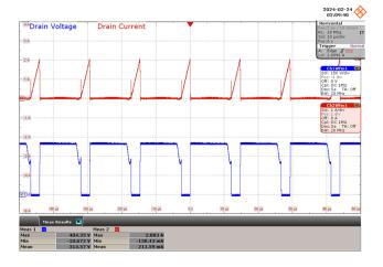
$\label{eq:Figure 60-230 VAC, 42 V LED Load.} \\ Upper: I_{DRAIN}, 1 \text{ A / div. (Max = 404.35 V)} \\ \text{Lower: } V_{DRAIN}, 150 \text{ V / div. (Max = 2.08 A)} \\ \text{Time Scale: } 10 \ \mu\text{s / div.} \\ \end{array}$
