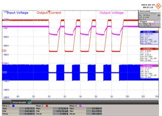
Figure 87 – 120 VAC, 42 V LED Load. 1 s On – 1 s Off. Upper:  $I_{OUT}$ , 1 A / div.  $V_{OUT}$ , 10 V / div. Lower:  $V_{IN}$ , 200 V / div., 2 s / div.
