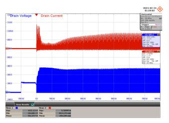
Figure 63 – 120 VAC, 42 V LED Load. Upper:  $I_{DRAIN}$ , 2 A / div. (Max = 422.13 V) Lower:  $V_{DRAIN}$ , 150 / div. (Max = 5.51 A) Time Scale: 100 ms / div.
