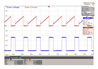
$\label{eq:Figure 58-100 VAC, 42 V LED Load.} \\ Upper: I_{DRAIN}, 2 A / div. (Max = 410.28 V) \\ Lower: V_{DRAIN}, 150 V / div. (Max = 3.93 A) \\ Time Scale: 10 \ \mu s / div. \\ \end{array}$
