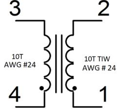
Figure 17 – CMC Electrical Diagram.
