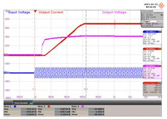
Figure 51 – 120 VAC, 42 V LED, Output Rise. Upper:  $V_{OUT}$ , 20 V / div,  $I_{OUT}$ , 1 A / div. Lower:  $V_{IN}$ , 300 V / div., 200 ms / div. Turn on Time: 652 ms
