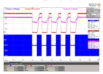
Figure 89 – 277 VAC, 42 V LED Load. 1 s On – 1 s Off. Upper:  $I_{OUT}$ , 1 A / div.  $V_{OUT}$ , 10 V / div. Lower:  $V_{IN}$ , 200 V / div., 2 s / div.
