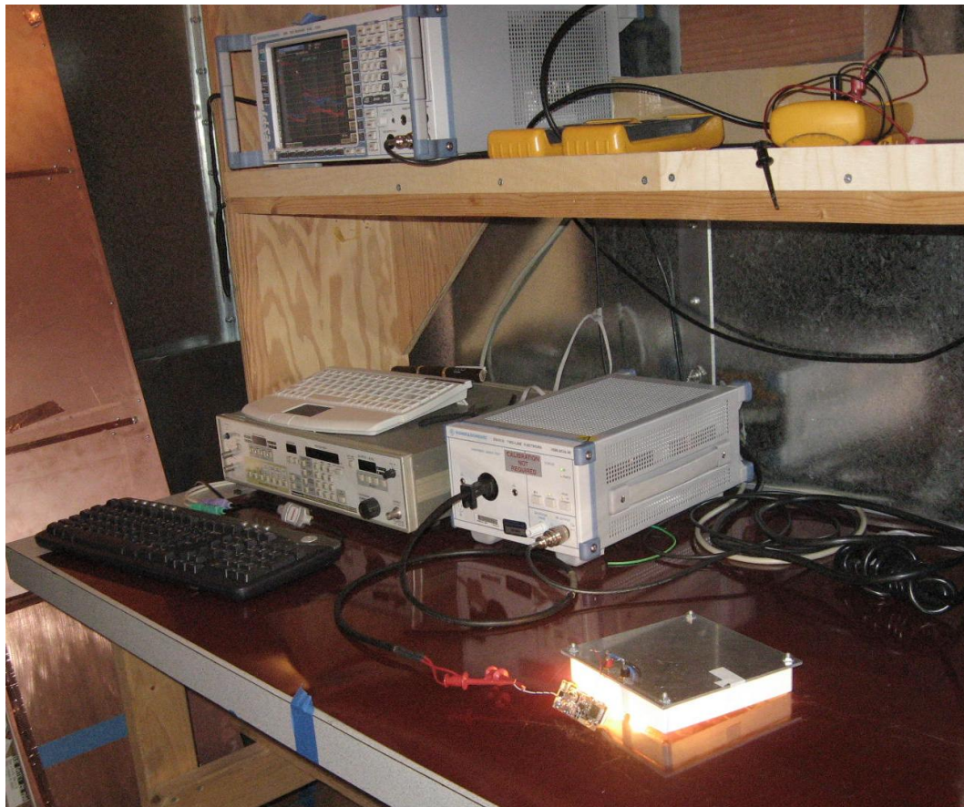
Figure 43 – Conducted Emissions Measurement Set-up.
