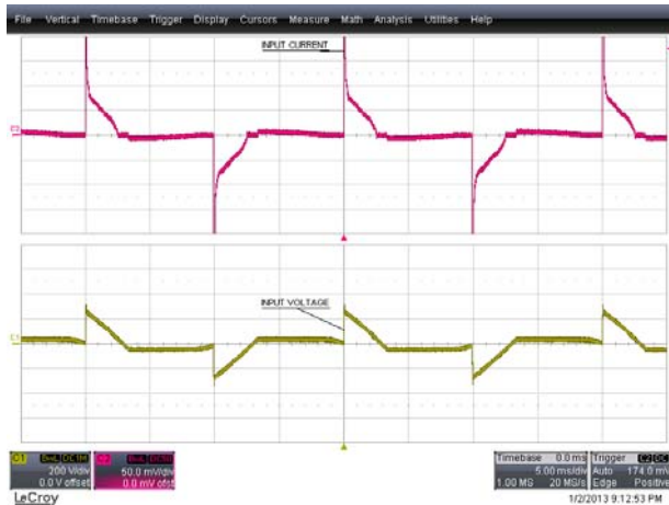
Figure 59 – 60° Conduction Angle. Upper: I_{IN} , 50mA / div. Lower: V_{IN} , 200 V, 5 ms / div.
