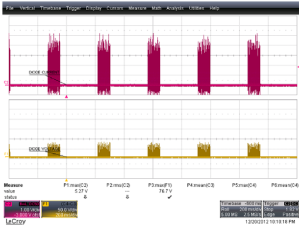
Figure 51 – 190 VAC, 50 Hz. Upper: I_{D7} , 1 A / div. Lower: V_{D7} , 50 V, 200ms / div.
