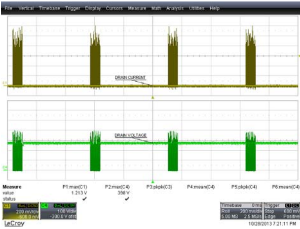
Figure 43 – 195 VAC, 50 Hz Output Short Condition. Upper: I DRAIN , 200 mA / div. Lower: V DRAIN , 100 V, 200 ms / div.
