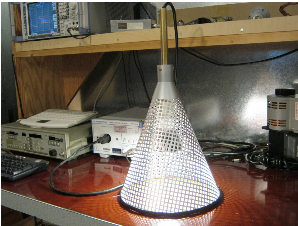
Figure 67 – EMI Test Set-up with the Unit and LED Load Placed Inside the Cone.
